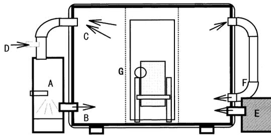
**Fig. 1** Arrangement in negative ion sauna room. A Shinki ionizer for production of negative ions, B duct introducing negative ion air, C exhaust air duct, D intake of fresh air, E wet sauna equipment, F duct for circulation of steam sauna, G transparent door
